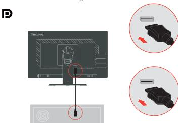
4. Connect one end of the HDMI cable to the monitor HDMI port and the other end to the computer if it has HDMI output terminal.
